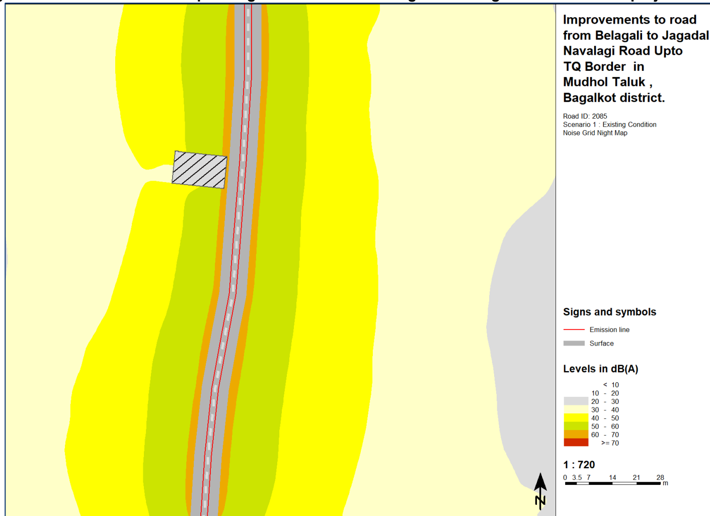
Figure 43: Scenario 1: Heat map for nighttime noise modelling for existing condition with no project scenario
