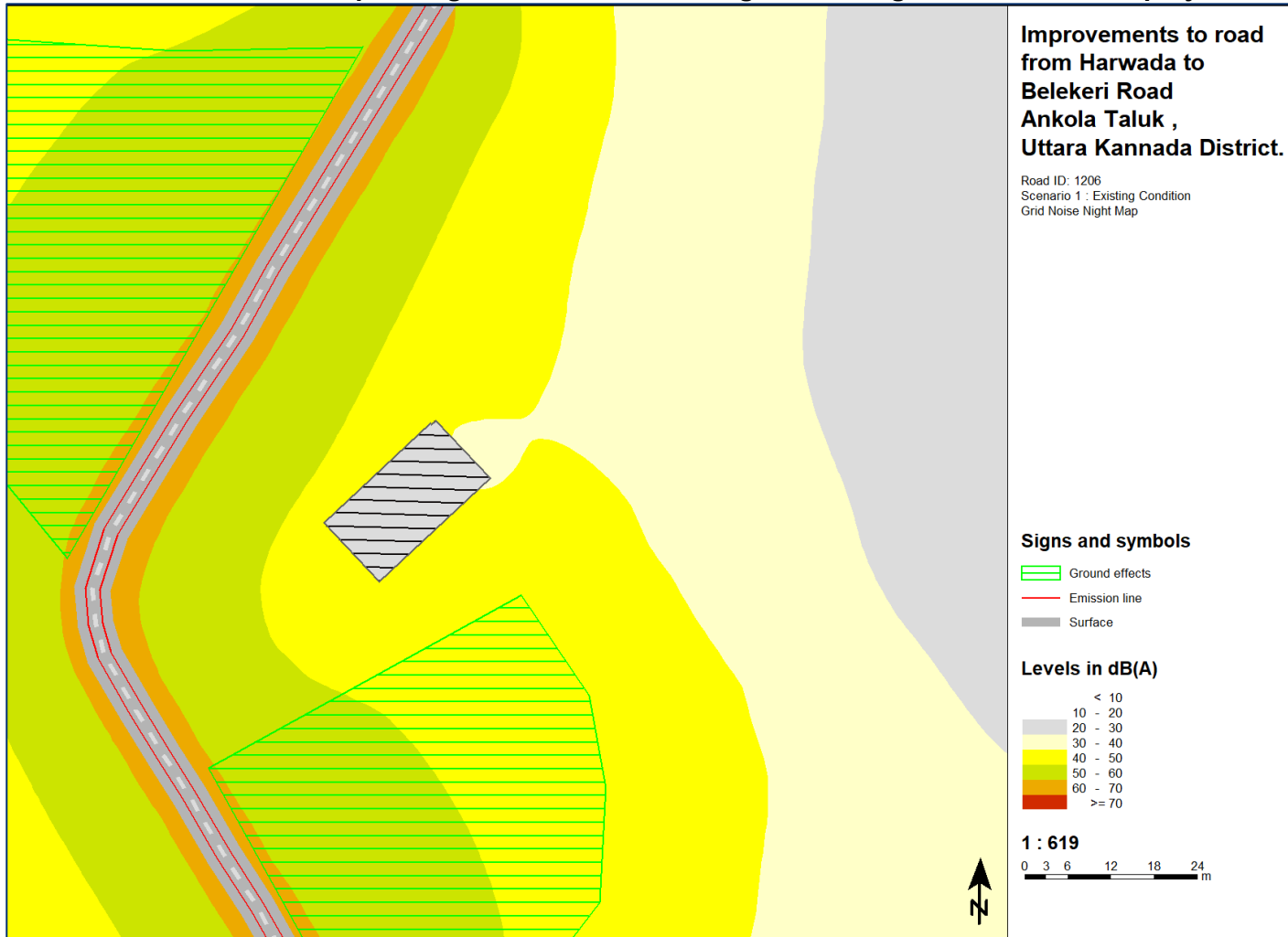
Figure 36: Scenario 1: Heat map for nighttime noise modelling for existing condition with no project scenario
