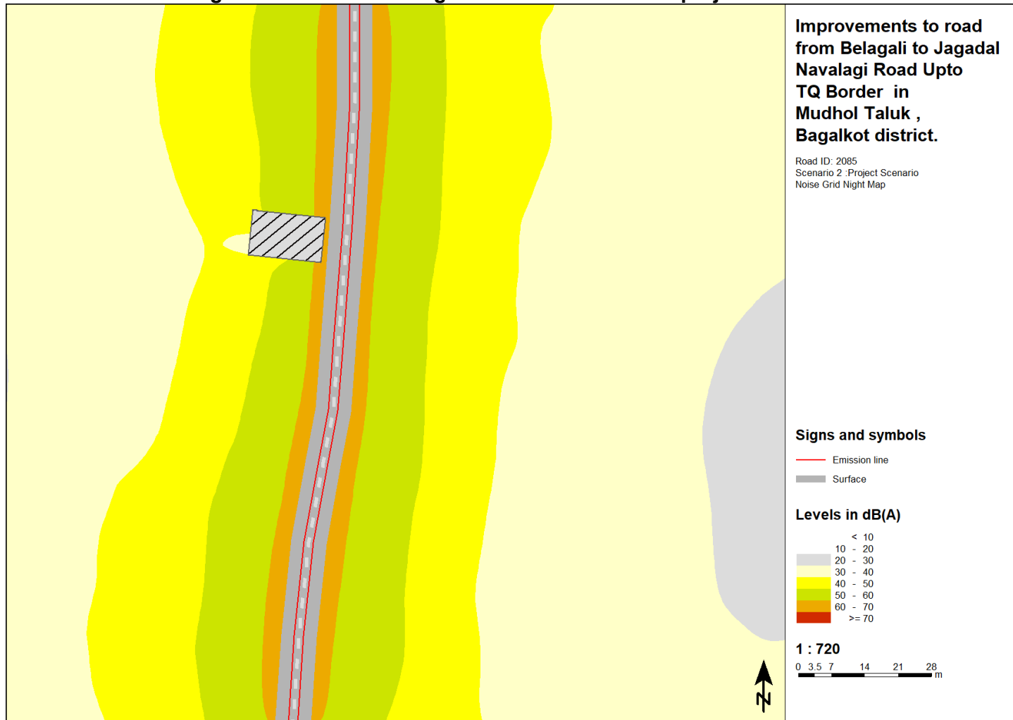
Figure 46: Scenario 2: Nighttime noise results for project scenario
